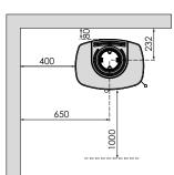
In order to avoid discolouration of painted and treated surfaces, TermaTech recommends the same distance from flammable materials as for non-flammable materials. This distance increases the convection itself around the stove and also eases cleaning. All distances relate solely to the distance of the stove from flammable materials. No account has been taken of national requirements for the use of stove flues or their distance from flammable materials.
