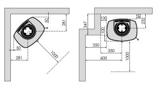
In order to avoid discolouration of painted and treated surfaces, TermaTech recommends the same distance from flammable materials as for non-flammable materials. This distance increases the convection itself around the stove and also eases cleaning. All distances relate solely to the distance of the stove from flammable materials. No account has been taken of national requirements for the use of stove flues or their distance from flammable materials.
