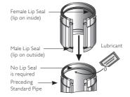
On 1-Piece Adjustable Pipe no lip seal is required on preceding standard pipe, as a male lip seal (once added) will ensure leakage performance. All lip seals to be added by installer.
