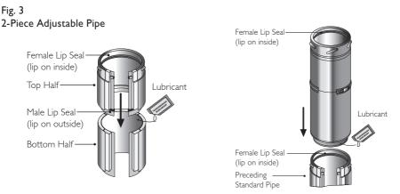
On 2-piece Adjustable Pipe a female lip seal is required on the preceding standard pipe to ensure leakage performance of the system. All lip seals to be added by installer.
