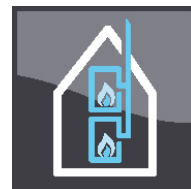
Decentralized multiple heating appliances connected to same chimney
