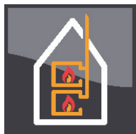
Decentralized multiple fireplaces connected to same chimney
