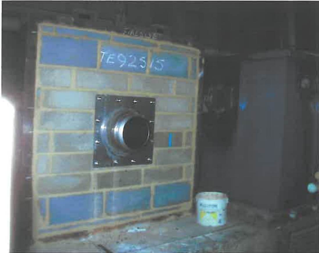
Plate 1 End of chimney and seal inside furnace before test
