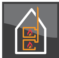
Decentralized multiple fireplaces connected to same chimney
