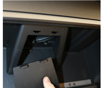
3. Twist the steel baffle as the pegs disengage from the housing to remove
