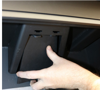
2. Removal is a simple process of pushing the top of the plate up which lifts the pegs clear of the housing
