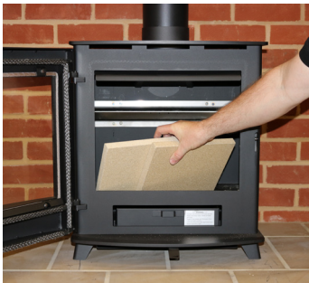
4. Remove the left hand side brick followed by the 2 rear bricks
